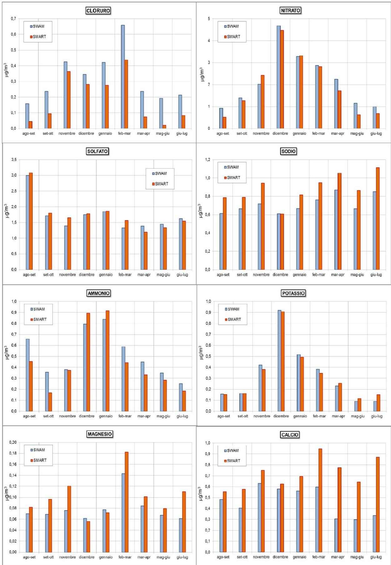
Figure 4: Concentration of inorganic ions: SMART SAMPLER vs. SWAM dual channel.
